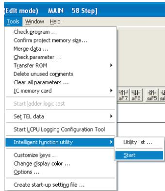
[Tools(工具)] - [Intelligent function utility(智能功能模块应用程序)] - [Start(启动)]
