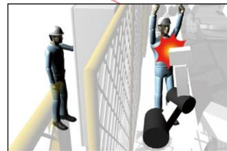
Starting a machine when an operator is within the safety fence can be dangerous.
