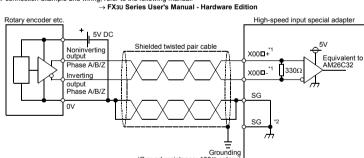
(Ground resistance: 100Ω or less) \*1 X00 indicates input number of the high-speed input special adapter.
