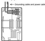
When connecting an input (only) extension block and an input/output extension block (e.g. FX2N-8ER) to the FX3U-1PSU-5V, supply the power of input circuit for them from the 24V DC service power supply of the nearest preceding main unit or powered extension unit.
