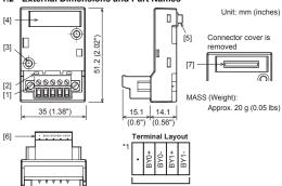
[1]Terminal block mounting screws [2]Output LED
